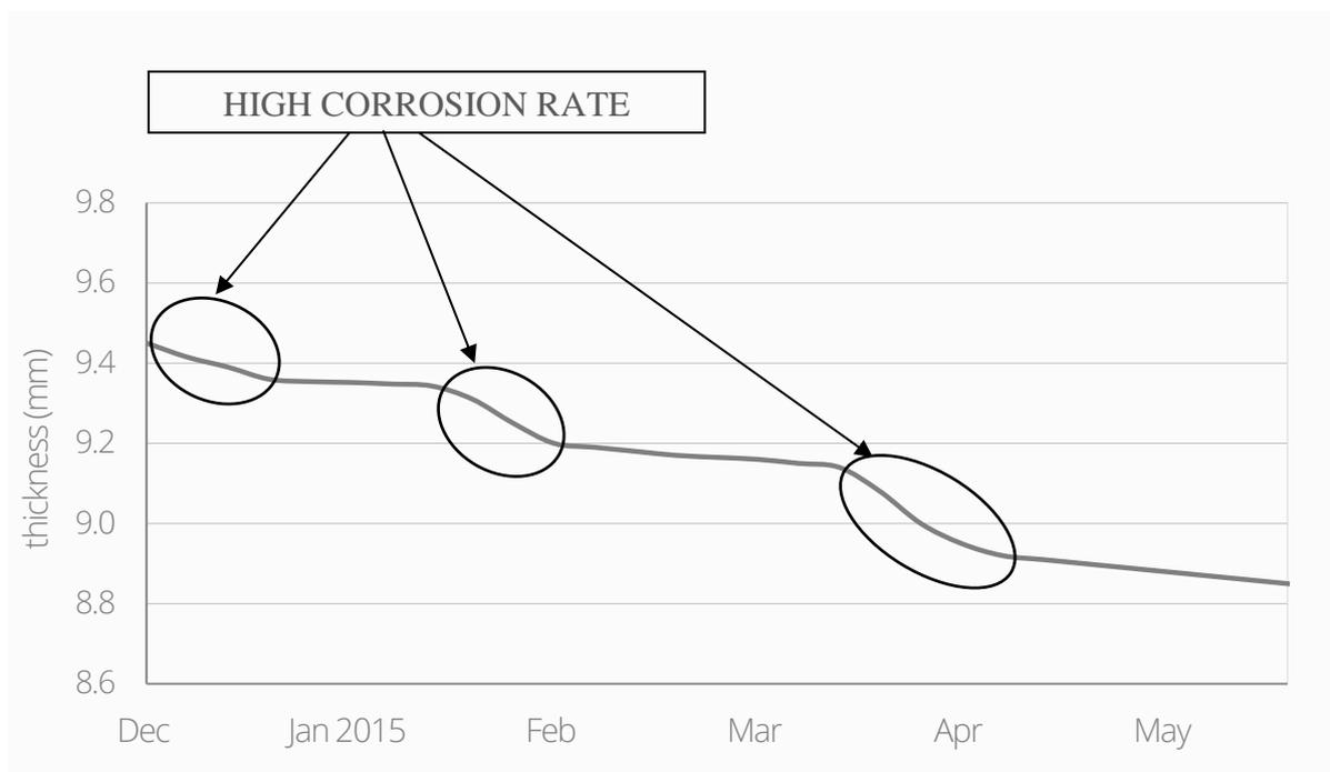
**Figure 6** SpotOn<sup>®</sup> U result at crude unit. Variable corrosion rate due to crude slate. Inhibitors dosage optimization possible using spotOn<sup>®</sup> U
