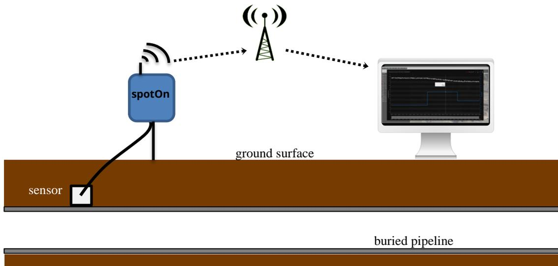
**Figure 2** SpotOn U installation and communication example
