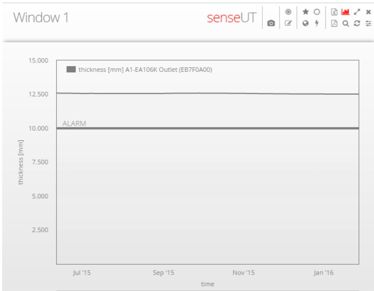
**Figure 5** Shieldcube thickness report window at SpotOn U installed at Aromatic unit in Figure 4
