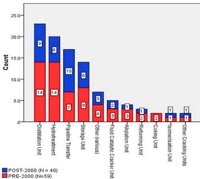
**Figure 3** Corrosion related accidents in the refining sector before year 2000 (in red) and after year 2000 (in Blue). Source @Corrosion related accidents in Petroleum refineries. JRC Scientific and Policy Report. European Commission
