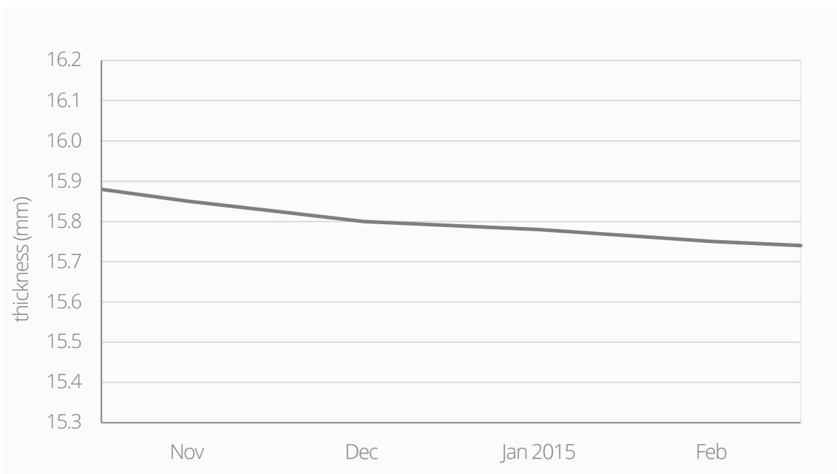
**Figure 7** SpotOn<sup>®</sup> U result at E&P facility. Inhibitor dosage optimization using output thickness data from spotOn<sup>®</sup> U
